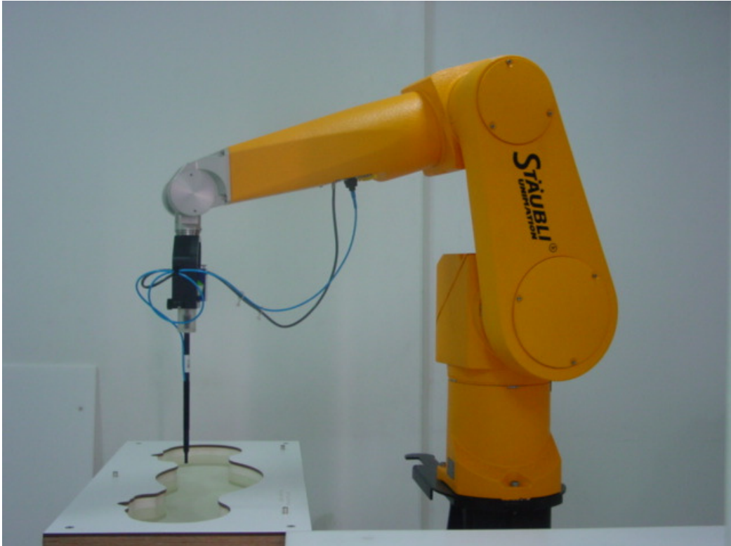
Picture 1: Specific Absorption Rate Test Layout
